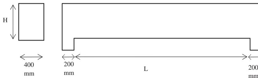
Fig. 2 Typical dimensions of the studied masonry beams.
