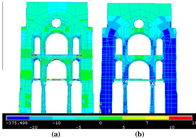
Fig. 14 Nonlinear analysis results by ANSYS (a) Sx and (b) Sz.
