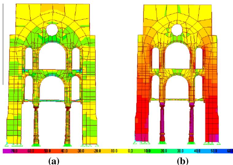
Fig. 13 Linear analysis results by SAP (a) Sx and (b) Sz.
